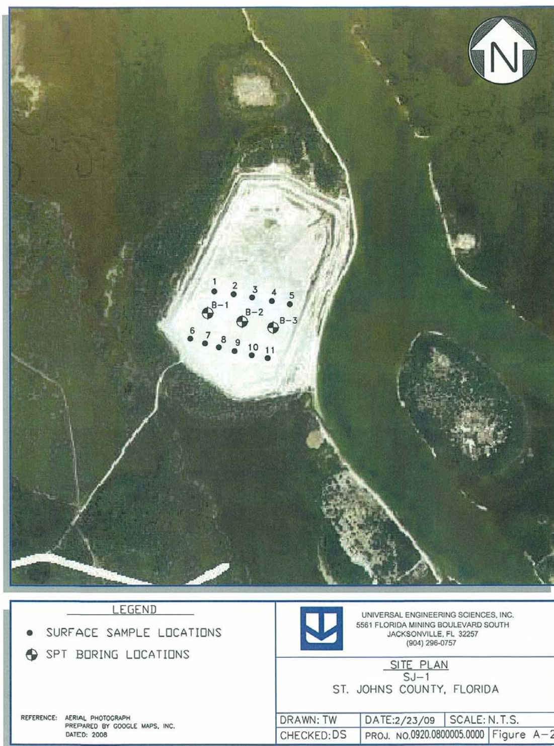
Figure 2.2 Borrow Area (FIND DMMMA SJ-1) Sampling Locations (Source: [UES, 2009])
