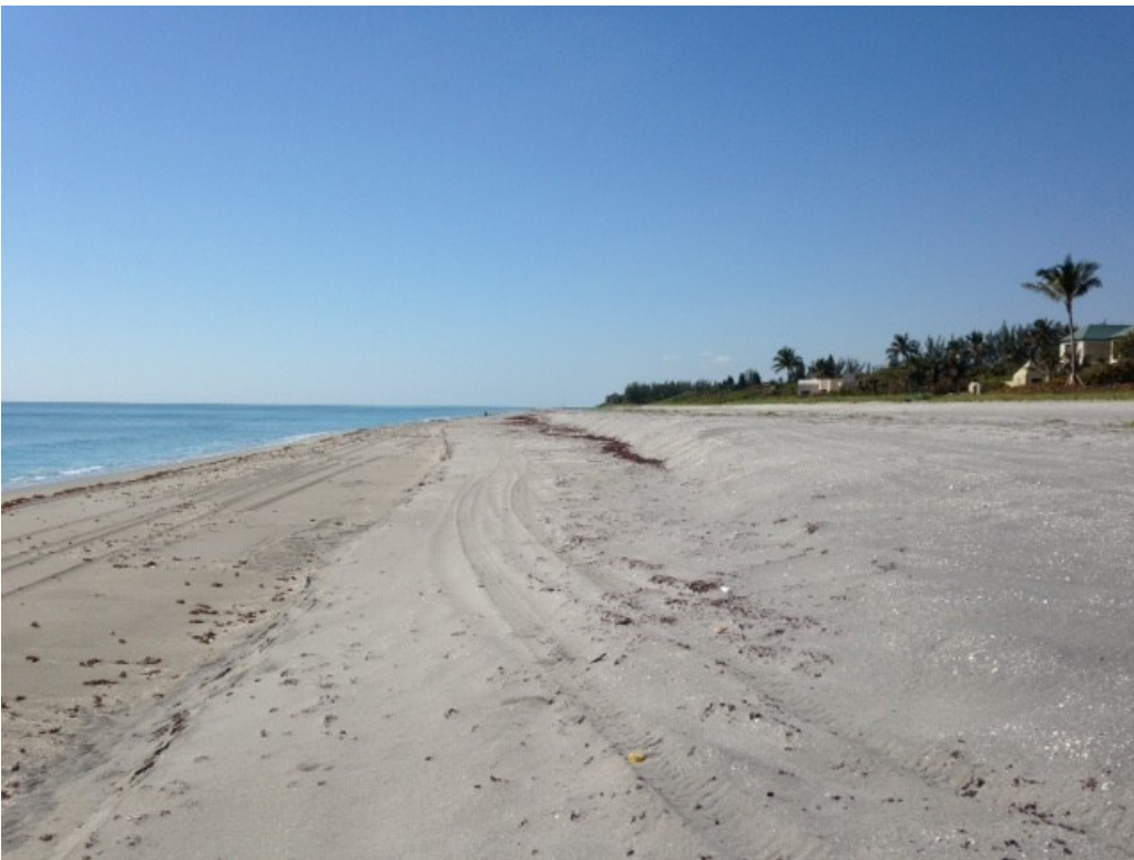
17. View looking south from ~R-104.5 seaward of 285 S. Beach Road, Jupiter Island (180-degree pan from Photo #16). A recently concluded JCP sand placement project has widened this beach considerably. Currently there is a low angle 2-4' scarp at mid-beach and further seaward.
