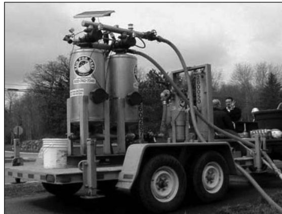
Sand media particulate filter (Source: http://www.spillcontainment.com )
