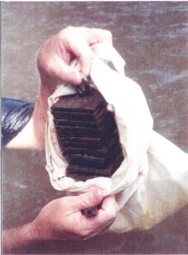
Hester-Dendy sampler collected in a draw string cotton bag.
