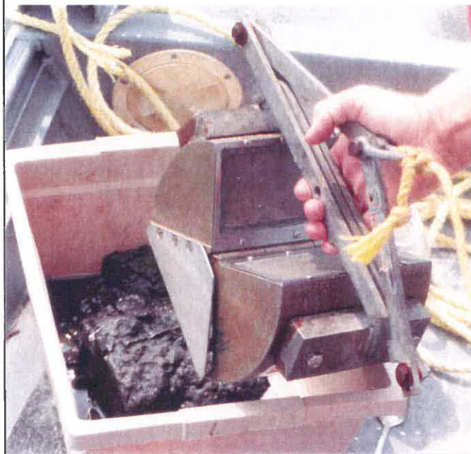
Collecting sediment with a petite Ponar dredge.
