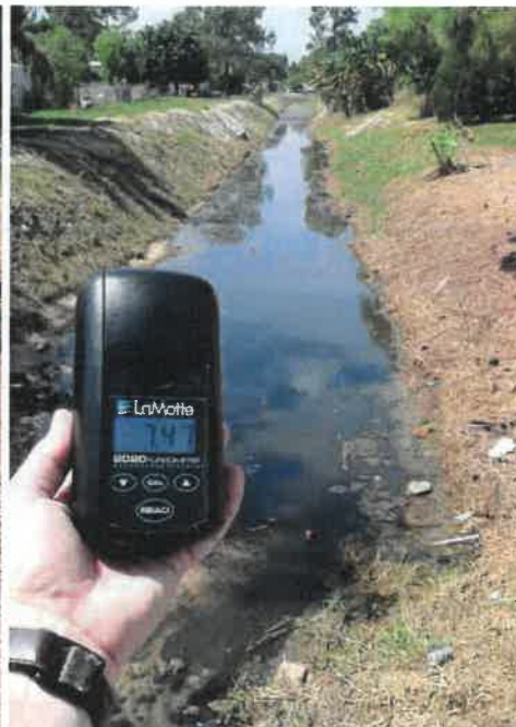
Clarity: The actual NTU value of the discharge water was read at about 7.5 NTU. The clarity and color of the water speaks for itself.
