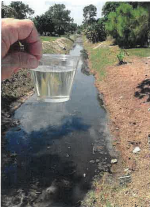
Clarity: The actual NTU value of the discharge water was read at about 7.5 NTU. The clarity and color of the water speaks for itself.
