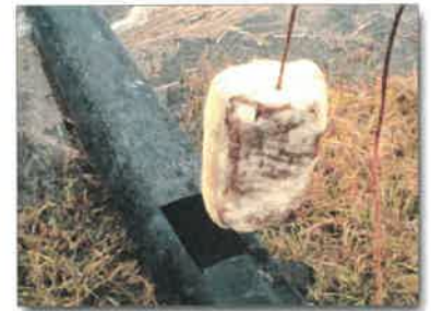
Figure 19. Polymer blocks inserted into pipes
