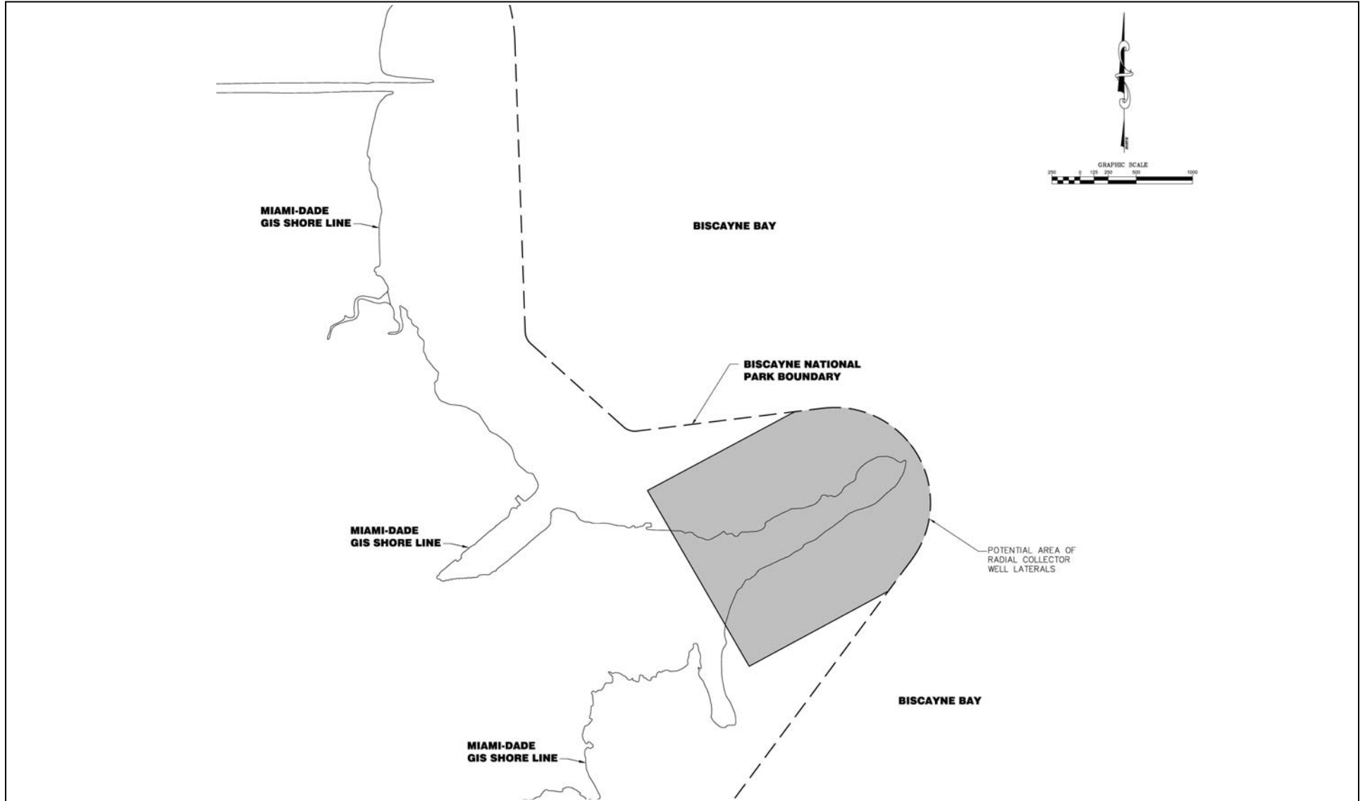
Figure 4.5-3 Potential Area of Radial Collector Well Laterals
