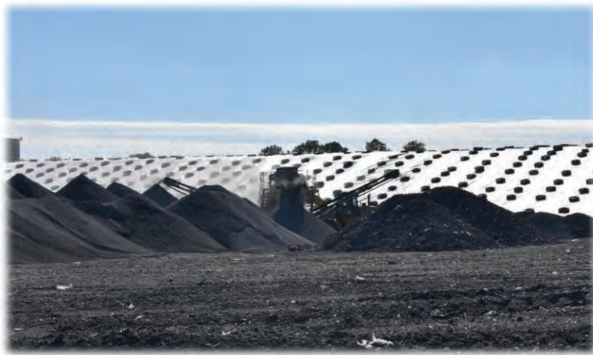
Figure 6-2 Segregated Aggregate Piles
