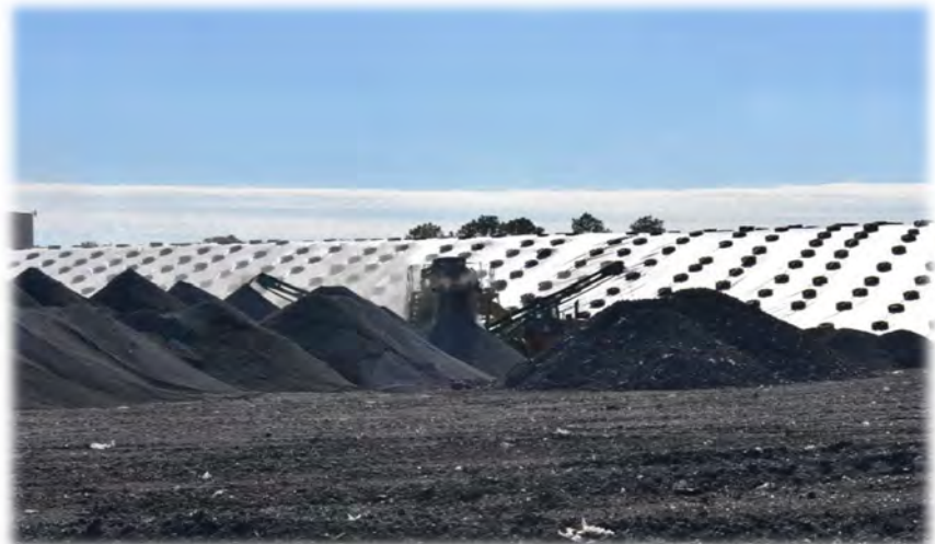
Figure 6-2 Segregated Aggregate Piles
