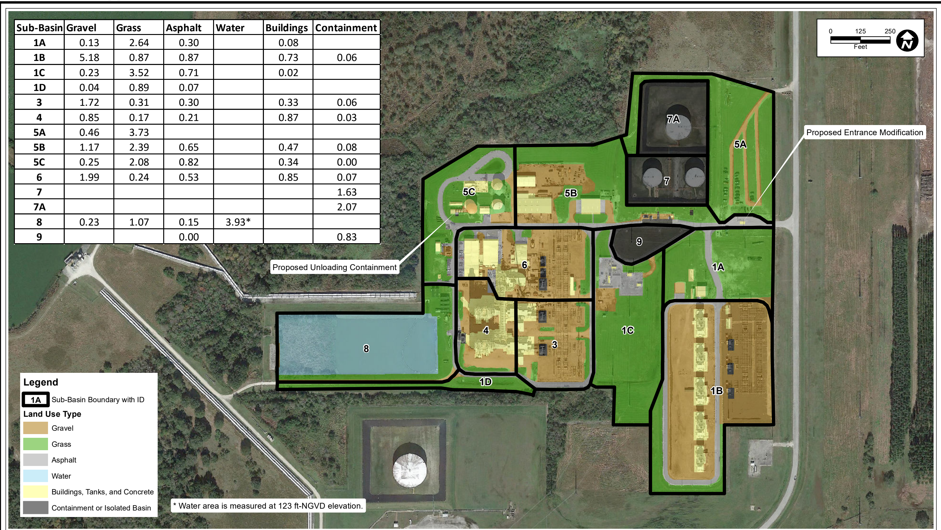
FIGURE 1. MGS DRAINAGE BASIN DELINEATION AND LAND COVER MAP
