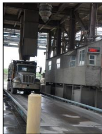
Unit 4 Fly Ash Loading for On-Site Disposal (foreground)
