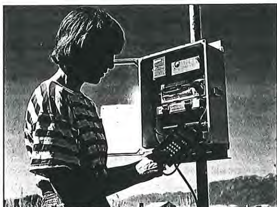
Programs can be entered or edited and system performance verified on-site with a CR10KD.
