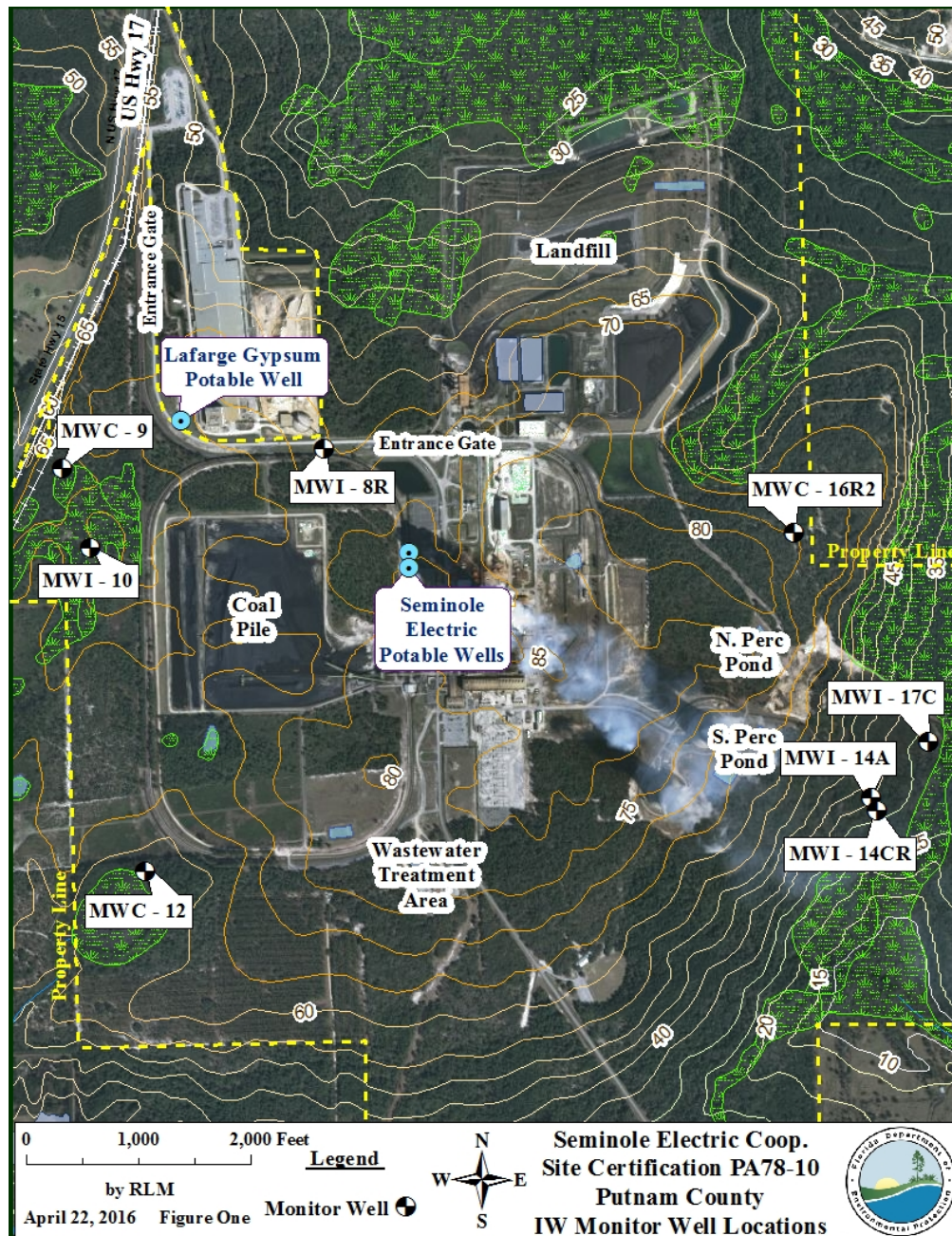
Figure 3. Industrial Wastewater Monitor Well Locations
