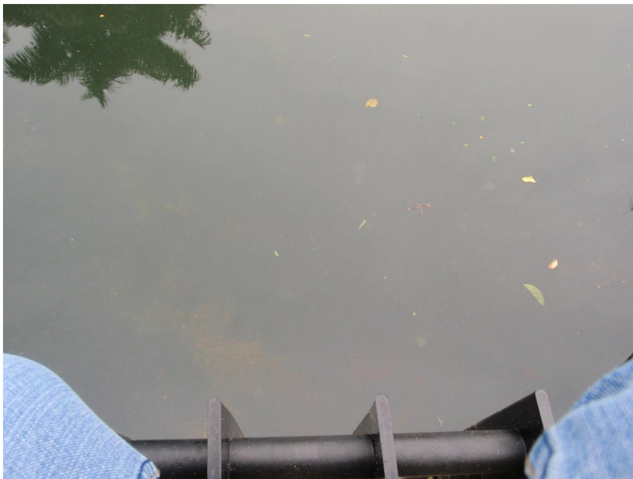
Figure 32. Solids and oils floating on surface water at a stormwater outfall from the VA Hospital building.
