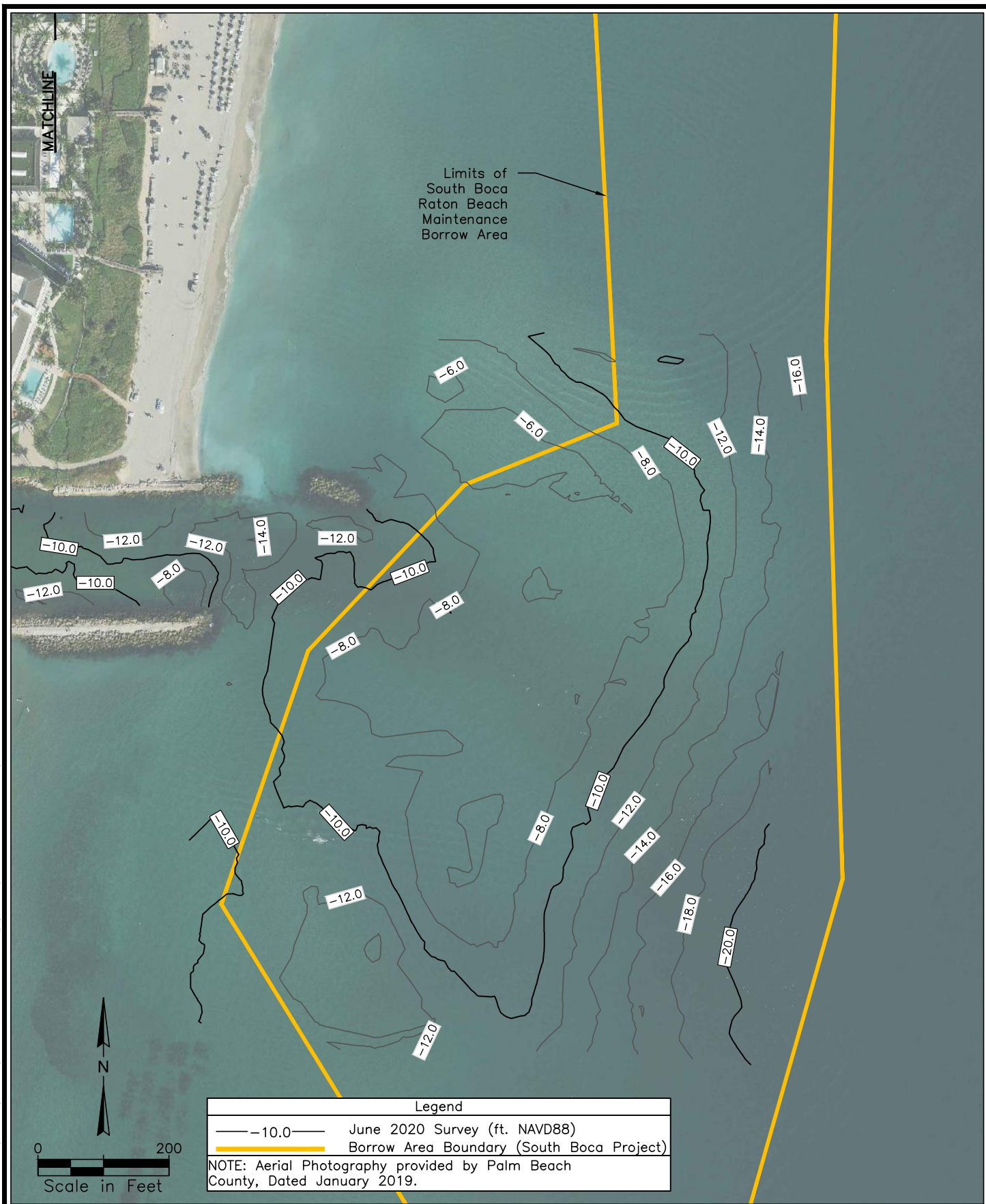
Figure 2b Hydrographic Survey (June 2020).
