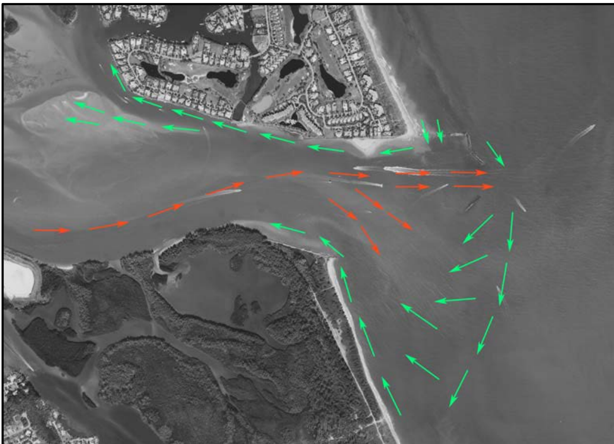
Figure 5. General flood and ebb sediment transport pathways (Ramsey et al, 2006).
