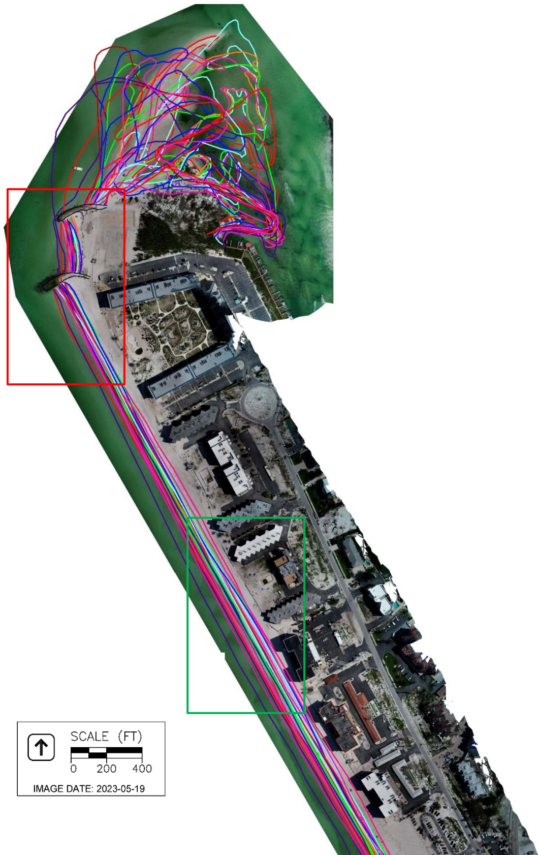
Figure 10 (continued on next page): Comparison of the Bonita Beach shoreline as observed from aerial photographs from 1994 through 2023. Each line represents the Bonita Beach shoreline from a different aerial photograph (ranging from 1994 to 2023). Figure adapted from Attachment B .
