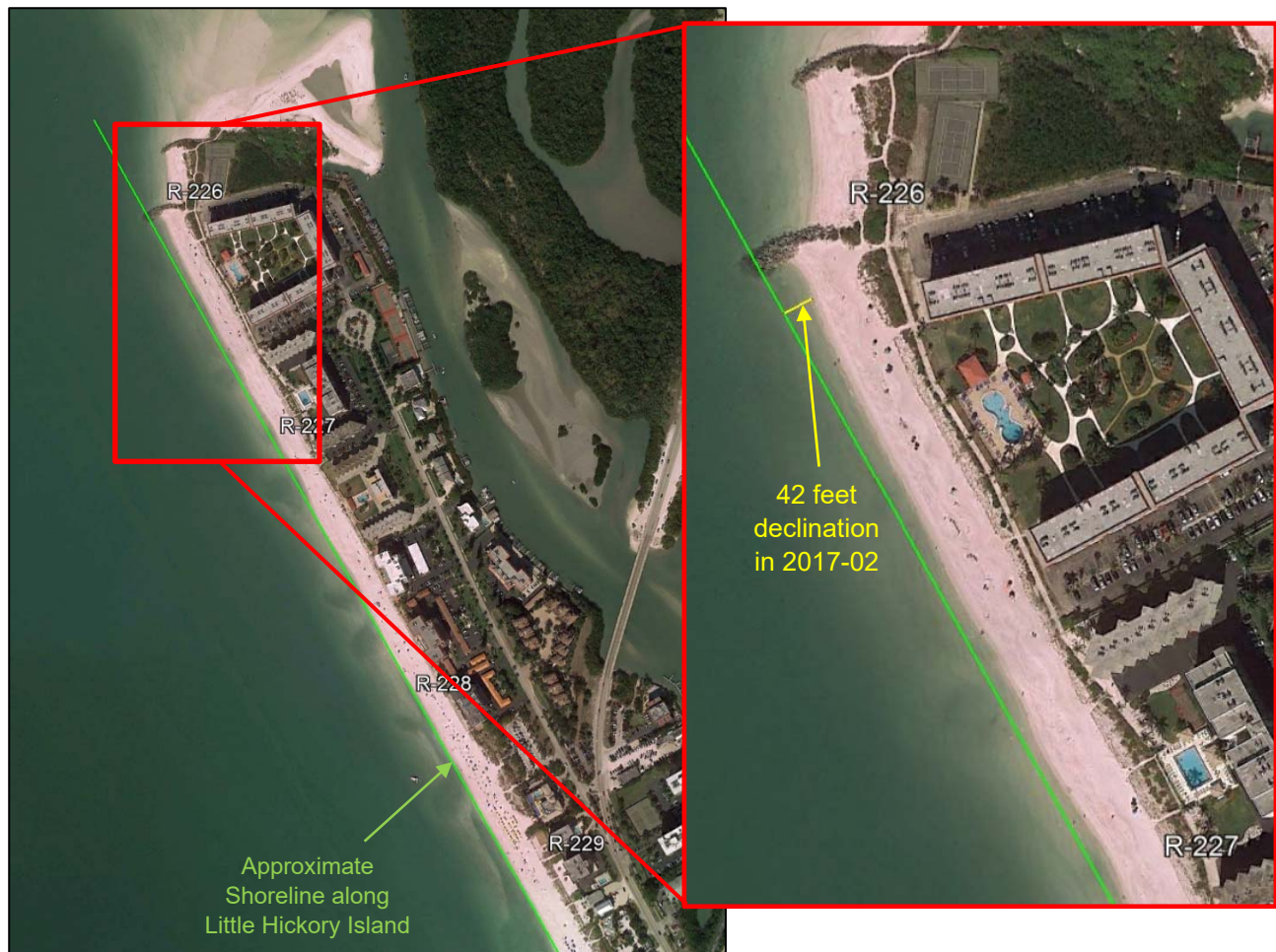
Figure 11: Aerial photograph of Little Hickory Island depicting a shoreline declination within 500–1,000 feet of the south groin. Aerial photograph dated February 2017 obtained from Google Earth. This landward declination of the shoreline, by 30 to 50 ft, is common to mostly all of the 2003-2023 aerial photographs.
