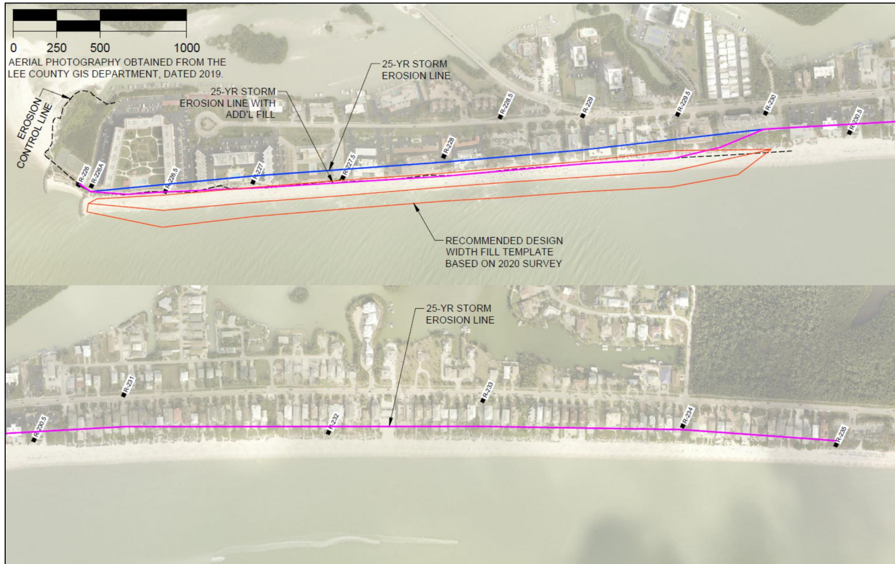
Figure 27. Erosion Predicted by SBEACH after 25-Year Storm Event for Recommended Fill Design.
