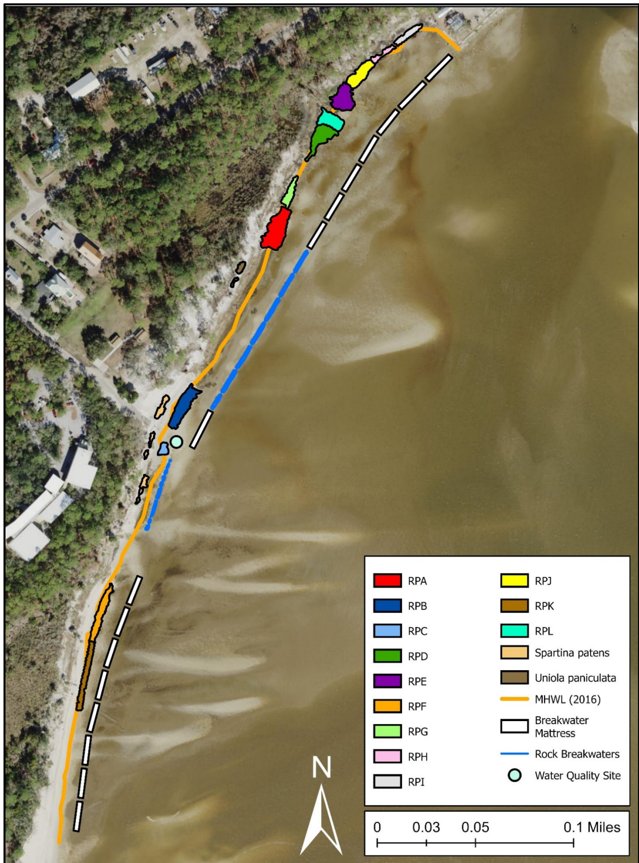
Figure 11. The Cat Point Living Shoreline as of April 2022. The second round of planting areas (2021 and 2022), surviving high marsh plantings from 2020 ( S. patens and U. paniculata ), constructed breakwaters, MHWL, old rock breakwater structures, and the water quality sampling site are included.
