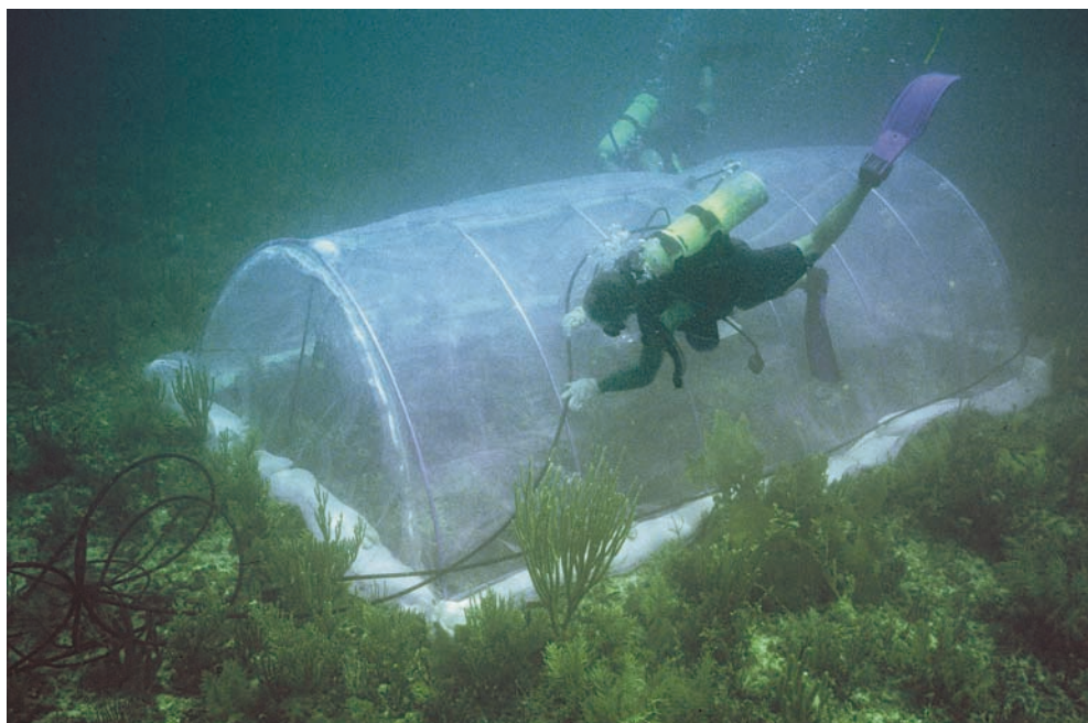
Fig. 1 The Submersible Habitat for Analyzing Reef Quality (SHARQ) is a large, portable benthic incubation chamber designed to isolate a mass of water over the underlying substrate. A flow-through analytical system enables continuous, 24-h monitoring of water chemistry resulting from benthic community processes
