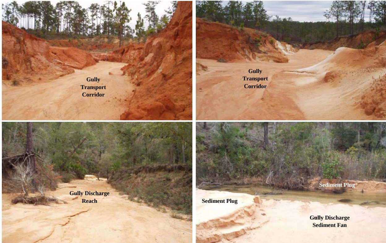
Figure 8. Northwest Florida Borrow Pit-Induced Gully Erosion and Stream Sedimentation
