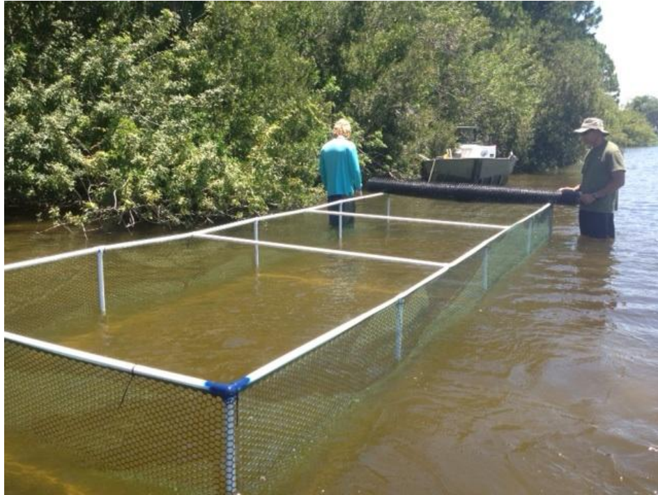
Figure 5. Herbivore exclusion cage (6m x 2m) being deployed May 2012 by FGCU researchers in the Caloosahatchee River and planted with Vallisneria americana (10 shoots/m 2 ).
