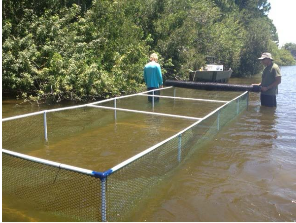
Figure 7. Herbivore exclusion cage (6m x 2m) being deployed May 2012 by FGCU researchers in the Caloosahatchee River and planted with Vallisneria americana (10 shoots/m 2 ).
