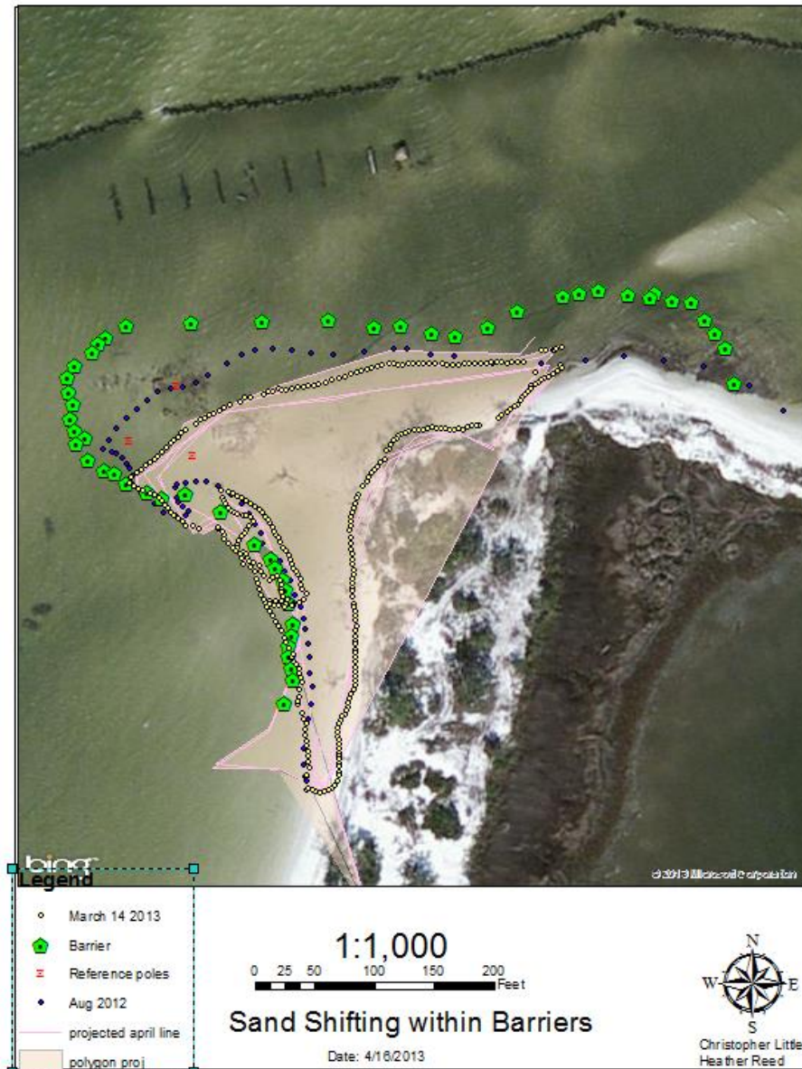
Figure 20-The barrier system (Green markers) was placed in May 2012. These markers are fixed reference points of anchoring for the barrier. The August 2012 after TS Issac points (blue points) show sand shifting and eroding back towards the peninsula. The March 20
