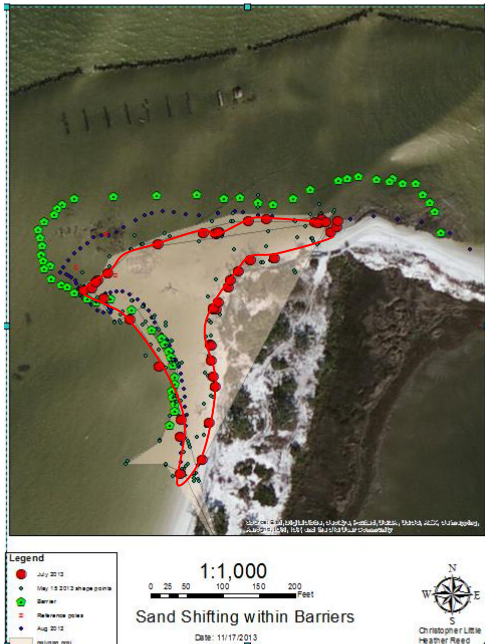
Figure 44: Sand shifting within the barriers of the fill site. The blue dots represent Aug 2012 and the red dots represent July 2013. The sand is shifting the south west and forming a small spit.
