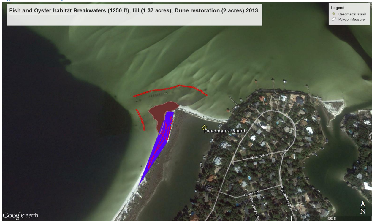
Figure 2: The footprint of proposed Dune restoration (blue) and Fish and Oyster habitat breakwater top units to be placed (red) and current fill location (brown) present at Deadman's Island. The red polygons within the blue shade represent north section of the historic dunes to be rebuilt.
