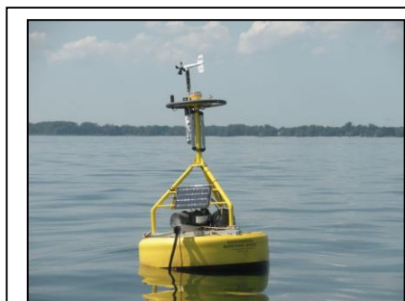
Figure 7. Continuous multi-parameter water quality monitoring buoy.
