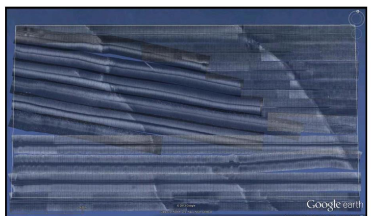
Figure 3. Over head view of the geo-referenced mosaic images from the side scan survey data.
