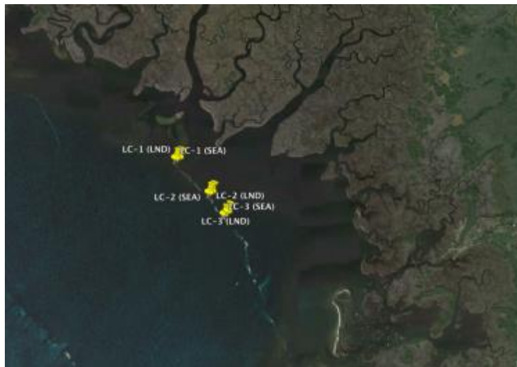
Figure 10. Locations of salinity recording instruments seaward and landward sides of Lone Cabbage reef.
