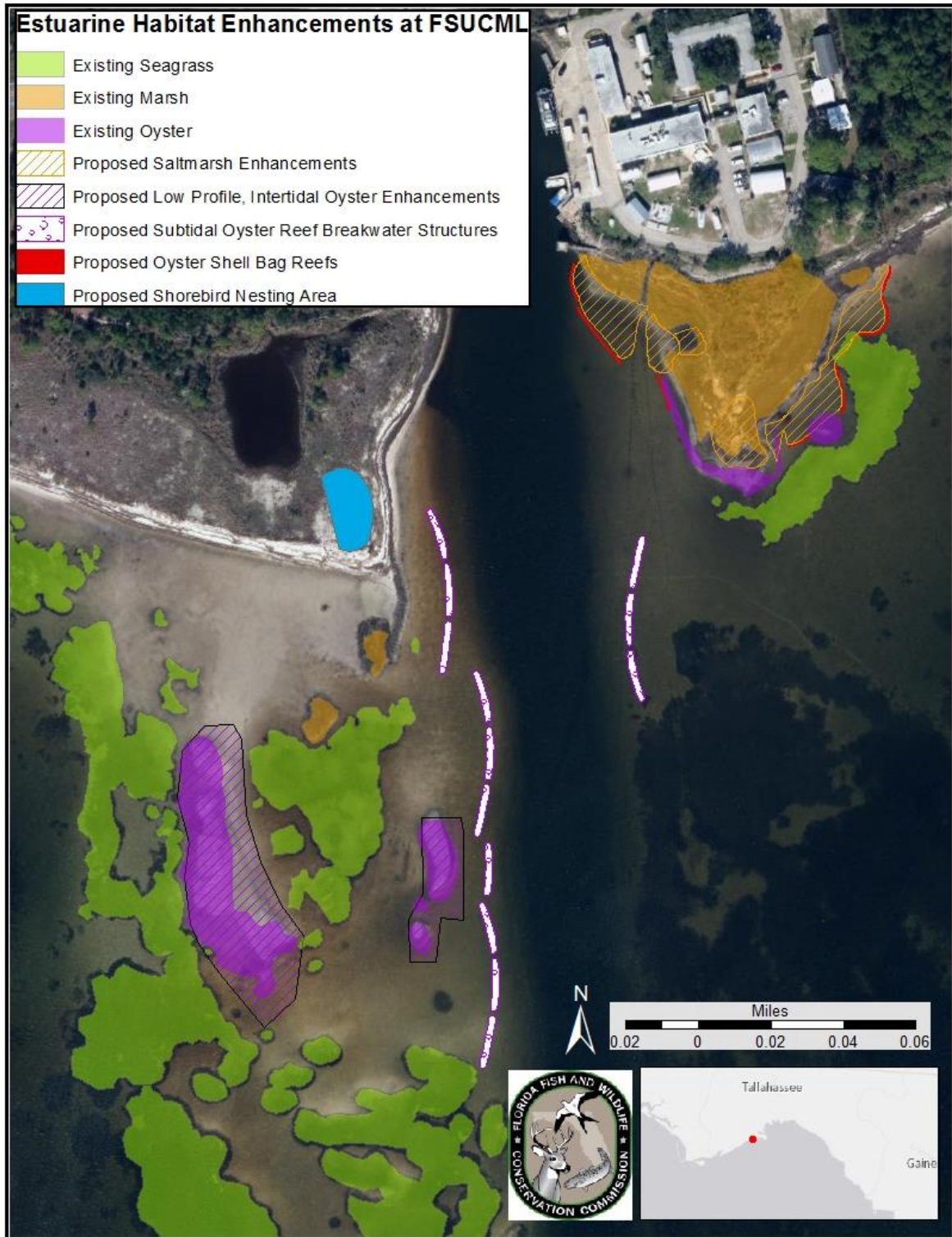
Figure 2. The Estuarine Habitat Enhancement at FSUCML project will create or enhance intertidal and coastal habitats including approximately: (1) 2 acres of saltmarsh; (2) 1.6 acres of oyster reef (including subtidal oyster reef breakwater structures, oyster shell bag reefs and low-profile, intertidal oyster habitat); and (3) 0.2 acre of shorebird nesting habitat.
