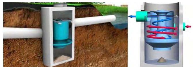
Figure ES- 4 Vortex Grit Removal Illustration ( www.hydro-int.com )
