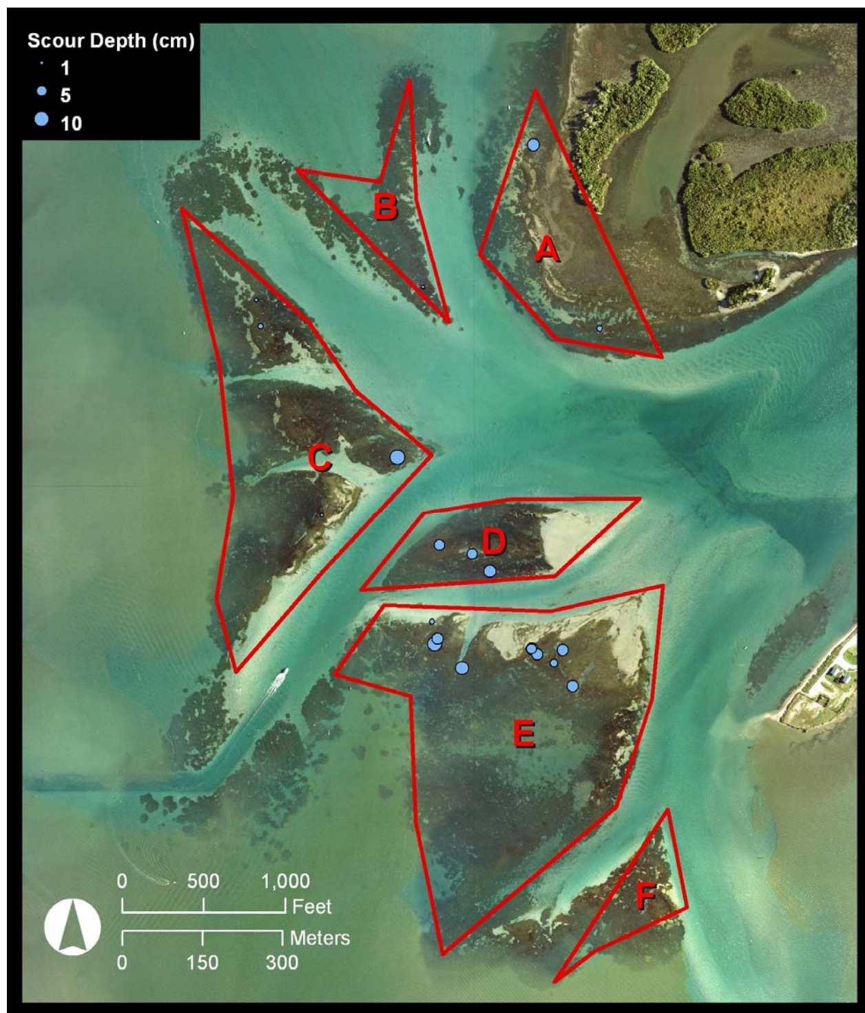
Figure 17. Scouring depth (cm) for Type III scarring observed within the mitigation area in 2010.
