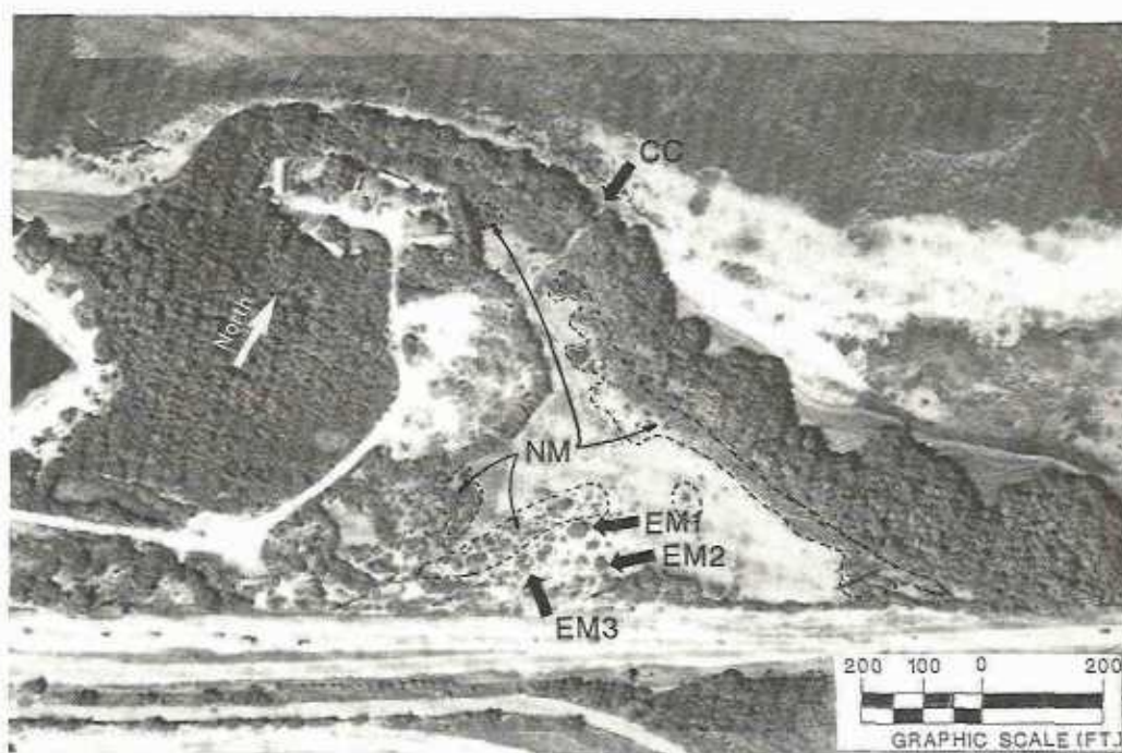
Figure 52. Vertical aerial photograph of Bahia Honda Lagoon taken February 12, 1991. CC indicates the location of the circulation cut made in March 1981. NM and dotted lines indicate the location of areas of natural mangrove recolonization, 1.35 acres (compare with above).
