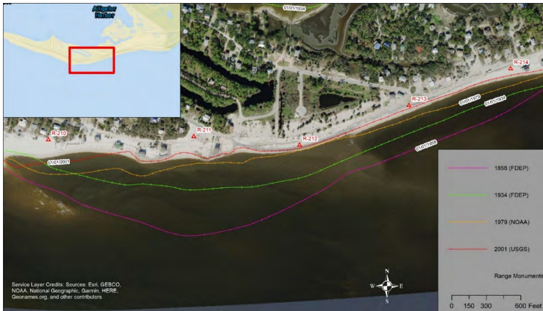
Figure 13: The segment of shoreline shown on this map has eroded significantly, as evidenced by historical map data. These lines show the approximate shoreline position over time, with the 1858 shoreline shown in purple (farthest from land) and the 2001 shoreline shown in red (closest to land). (USGS n.d.[b])
