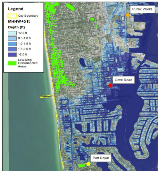
Figure 3. Sea Level Rise Exposure of Naples Stormwater Pump Stations. Area south of the pier shows predicted sea level rise associated flooding in historic Old Naples.
