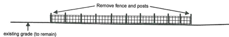
TYPICAL LONG SECTION LOOKING N or W
