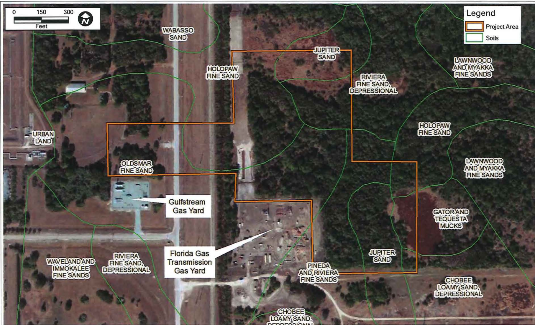
FIGURE 4. SOILS RIVIERA LATERAL MARTIN GAS YARD
