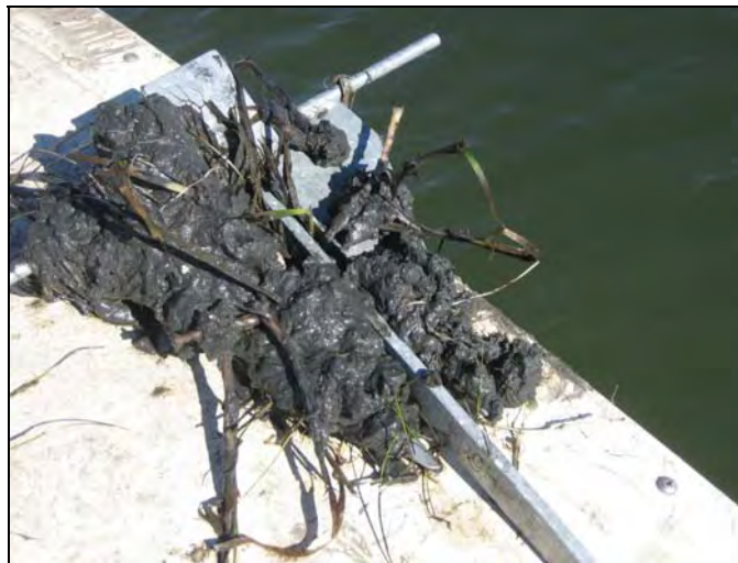
Figure 11. The anchor would occasionally capture vegetation samples in seagrass beds when rake sampling did not.
